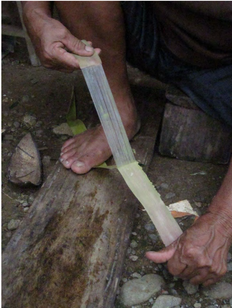
Fig. 2. Extracting liniwan 2014, the innermost fiber of the leaf of the pineapple plant, Barangay Fulgenzio del Norte, Aklan, Panay, the Philippines
